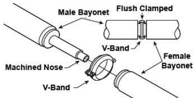
Note: Bayonets that are cold (that have been in service) should be warmed to close to room temperature for easier disengagement. To do this, the VJP must be drained of liquid and allowed to warm up for approximately 24 hours before attempting disengagement. Contact Midwest Cryogenics if a more rapid time is necessary.
