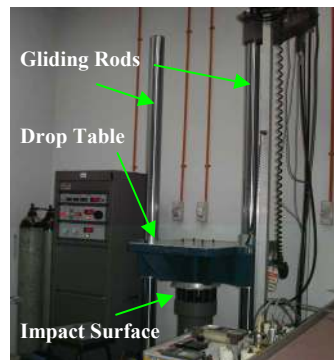
Fig 1. Lansmont Model 65/81 Drop Impact Tester.
